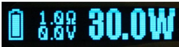
The DNA 30D has a small .69" diagonal blue OLED screen. The screen is attached to the main board by a flexible cable, allowing freedom in the design of your device. Please use caution when handling the screen and design the device so that the cable will be secured or strain relieved in operation. The normal and special operating modes shown on the display are discussed below.
