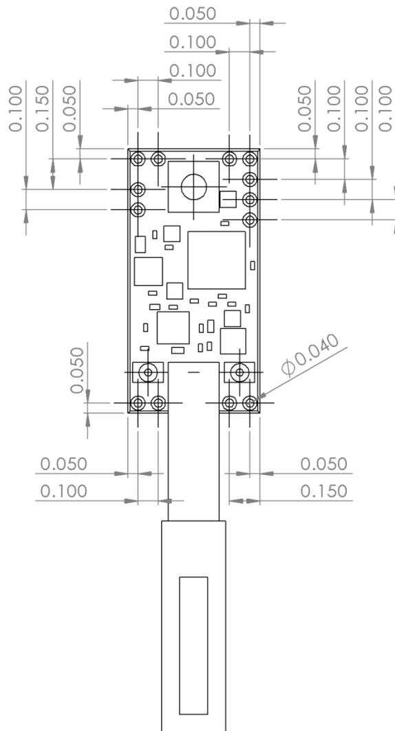
The mounting holes for the DNA 30D are .100" pitch and .040" diameter. It can be wired in directly using soldered connections, or socketed with .1" hardware.
