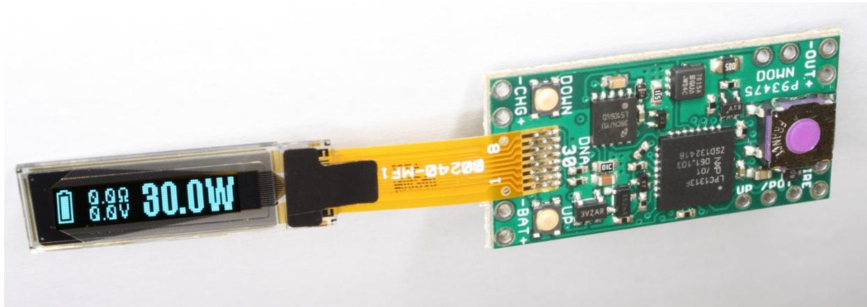
The DNA 30D is a power regulated digital switch-mode DC-DC converter for personal vaporizers. It features a small OLED display, analog or digital user controls, onboard buttons and synchronous rectification for maximum battery life and minimal heat generation.
